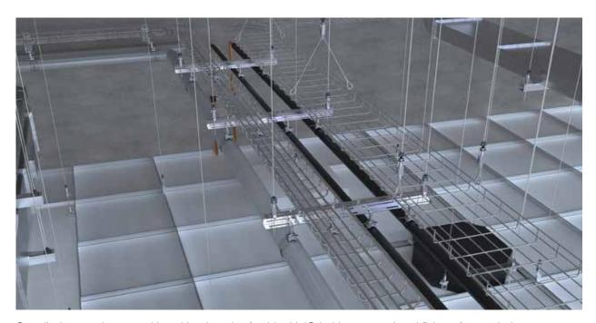
Supplied as ready-to-use kits with a length of cable, UniGrip Hanger, and end fixing of your choice.
