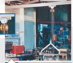
**Die-Handling Trolley System** This system makes use of back-toback Unistrut channel track sections and ball-bearing trolleys to produce an overhead support structure with movement in two directions.
