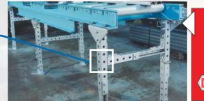
**Conveyor Support** This conveyor support structure, made entirely from Telestrut components, is engineered to provide infinite adjustment in both width and height, making it adaptable to a wide range
